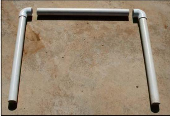
To assemble the base, glue a right-angle pipe fitting to 2 of the cut pipes and lay out these assemblies and a third pipe as shown in the photo on the left.
