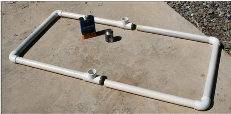
To complete the base assembly remove the assembly that was loose-fitted and glue the two parts together as shown on the left.
