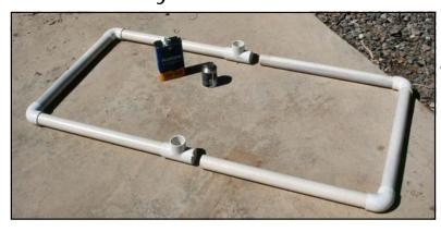
To complete the base assembly remove the assembly that was loose-fitted and glue the two parts together as shown on the left.
