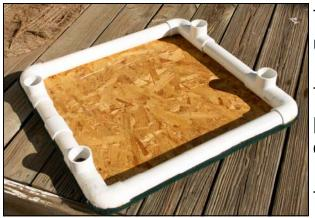
The top is assembled in a similar way using the remaining lengths of PVC.
